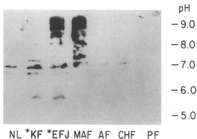
Figure 8. Western blot analysis of the binding of radiolabeled DNA to serum samples from family 2. Lane NL; serum from a normal control. Lanes K.F. and E.F.J.; serum from SLE patients. Lanes M.A.F., A.F., C.H.F., and P.F.; serum from unaffected family members. E.F.J. and M.A.F. show DNA-binding immunoglobulins.
