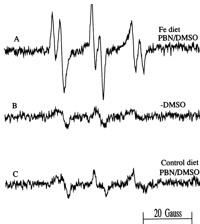
Figure 1. (A) ESR spectrum of radical adducts detected in the bile of rats fed the high-iron diet for 10 weeks collected 40 min after intraperitoneal administration of PBN (70 mg/kg) dissolved in DMSO (1 ml/kg). Bile samples (~400 \mu l) were collected into a 30 mM 2,2'-DP (25 \mu l/100g of rat weight). (B) Same as in A, but rats were not administered DMSO. (C) Same as in A, but rats were fed the regular control diet. Instrumental conditions: microwave power, 20 mW; modulation amplitude, 1.33 G; time constant, 1 s; scan time, 16 min.
