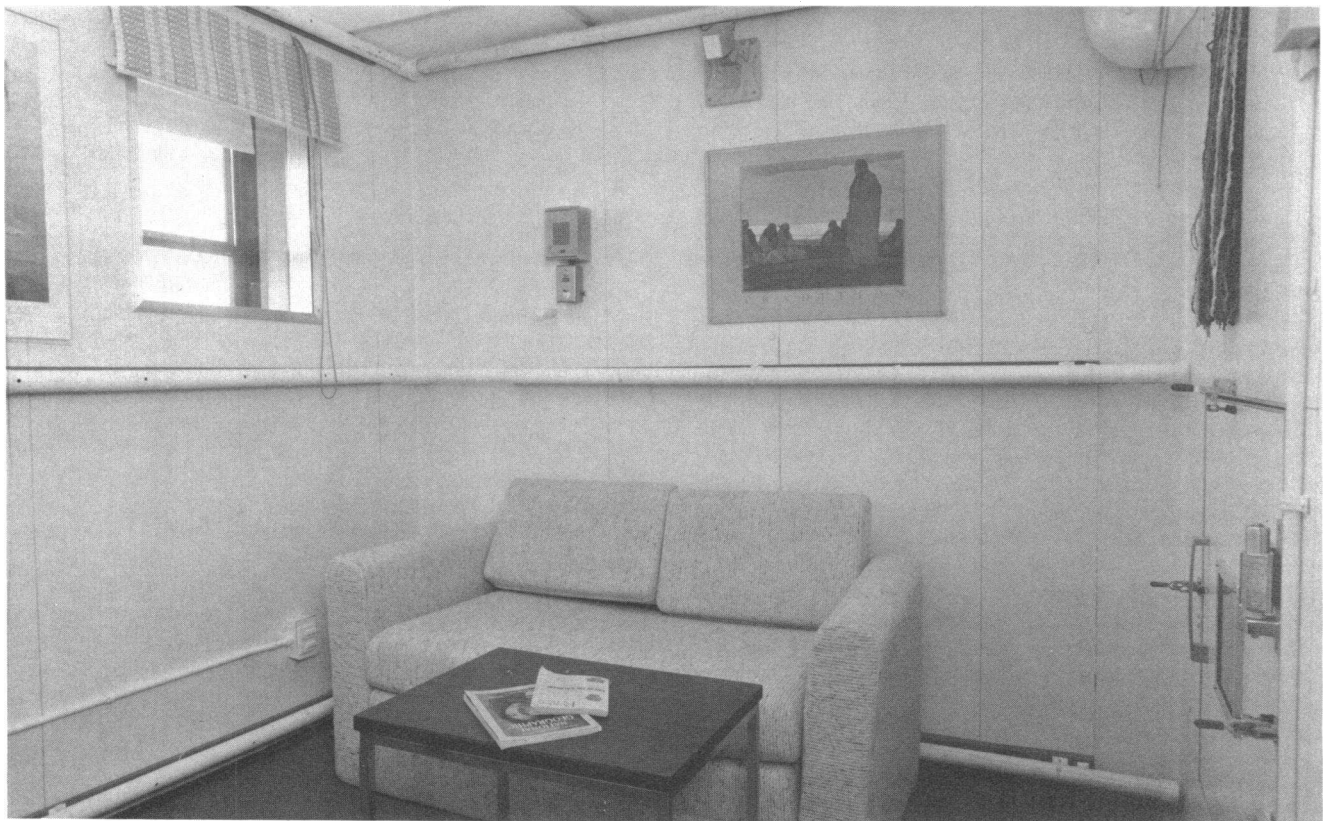
Figure 1. The Phoenix respiratory chamber (19,000 liter) based on the principle of open-circuit indirect calorimetry. Note in the upper photograph the radar system located above the mirror and in the lower photograph the air sampling lines disposed on two walls at three different levels.
